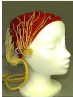
It is possible to measure a person's dominant brainwave frequency in a laboratory by using an 'Electro-Encephalogram', or EEG.
